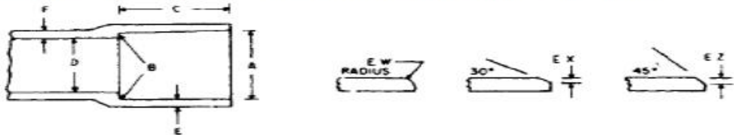
Tapered Sockets for PVC Pipe Fittings, Schedule 80, in. (mm) A
